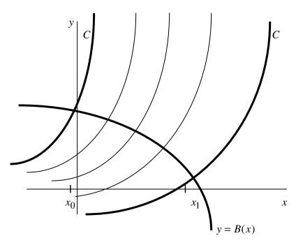
The solution exists in the region bounded by the two characteristic lines, labelled C; data is given on the line y = B(x), between  $x = x_0, x_1$ .
