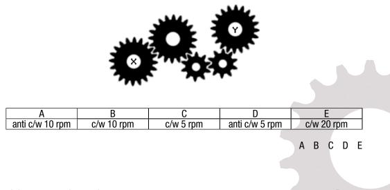
7) If gear X turns clockwise at a constant speed of 10 rpm. How does gear Y turn?
