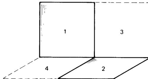
Figure 10.12 Radiation between two offset perpendicular squares.
