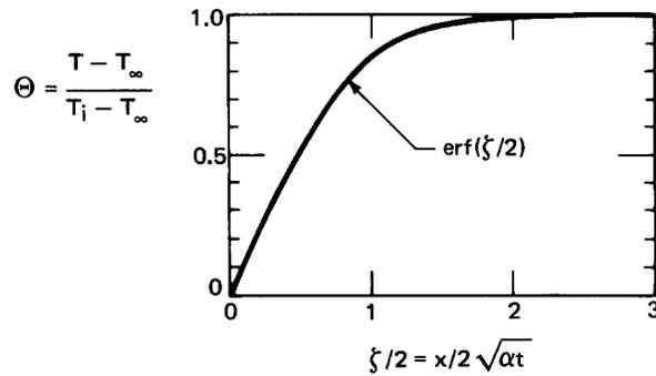
**Figure 5.15** Temperature distribution in a semi-infinite region.
