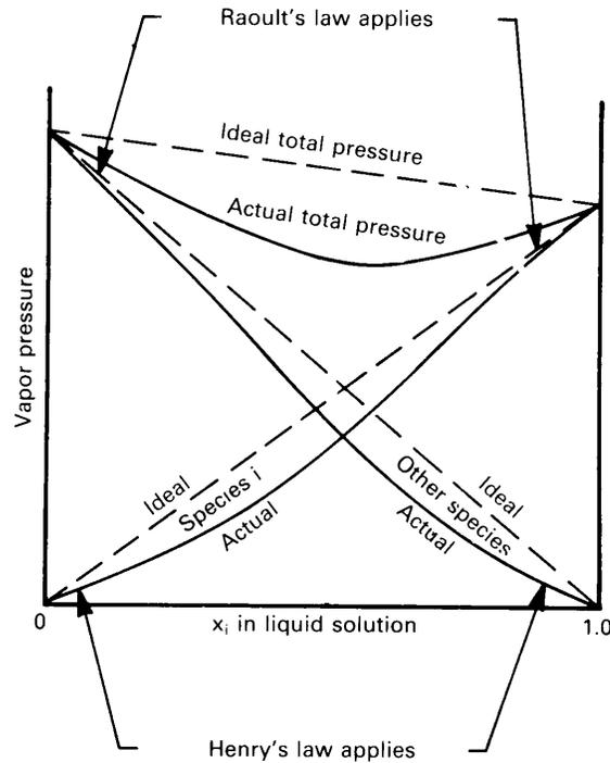
**Figure 11.10** Typical partial and total vapor-pressure plot for the vapor in contact with a liquid solution, illustrating the regions of validity of Raoult's and Henry's laws.
