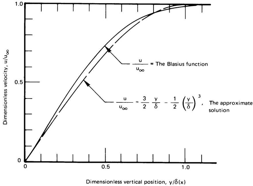
**Figure 6.11** Comparison of the third-degree polynomial fit with the exact b.l. velocity profile. (Notice that the approximate result has been forced to  $u/u_\infty = 1$  instead of 0.99 at  $y = \delta$ .)
