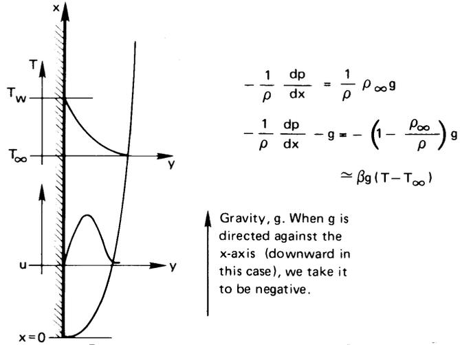
**Figure 8.2** Natural convection from a vertical heated plate.
