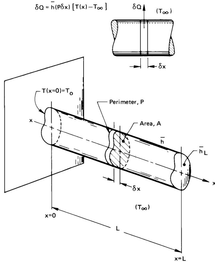
Figure 4.8 The analysis of a one-dimensional fin.
