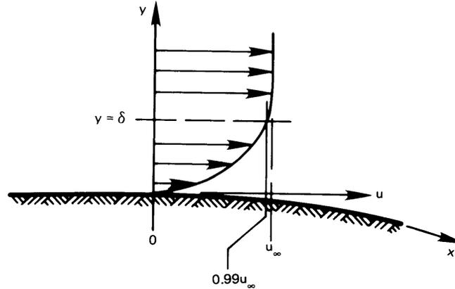
**Figure 6.1** A boundary layer of thickness  $\delta$ .
