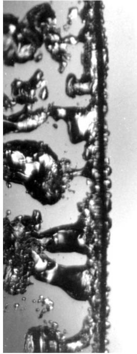
3.45 cm length of 0.0322 cm diam. wire in methanol at 10 earth-normal gravities.  $q=1.04 \times 10^6 \text{ W/m}^2$
