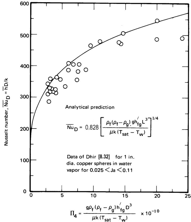
**Figure 8.10** Correlation of the data of Dhir [8.32] for laminar film condensation on spheres at one value of  $Pr$  and for a range of  $\Pi_4$  and  $Ja$ , with properties evaluated at  $(T_{sat} + T_w)/2$ . Analytical prediction from [8.33].
