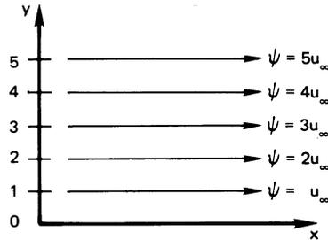
**Figure 6.8** Streamlines in a uniform horizontal flow field,  $\psi = u_\infty y$ .
