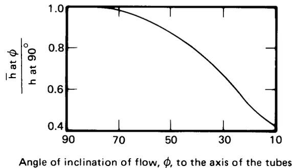
**Figure 7.16** Correction for the heat transfer coefficient in flows that are not perfectly perpendicular to heat exchanger tubes [7.28].
