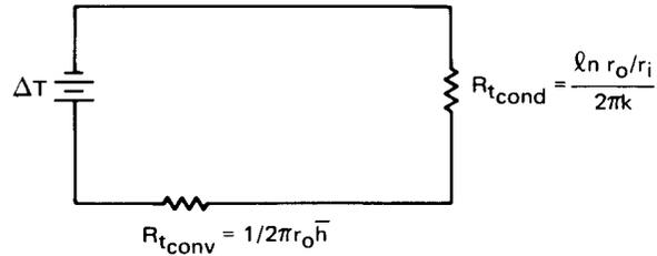
**Figure 2.14** Thermal circuit with two resistances.
