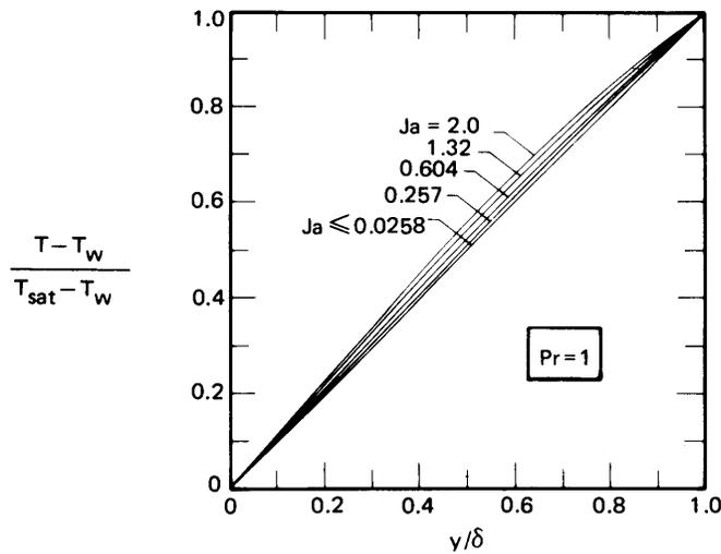
**Figure 8.12** Results of the exact b.l. analysis of laminar film condensation on a vertical plate [8.36].
