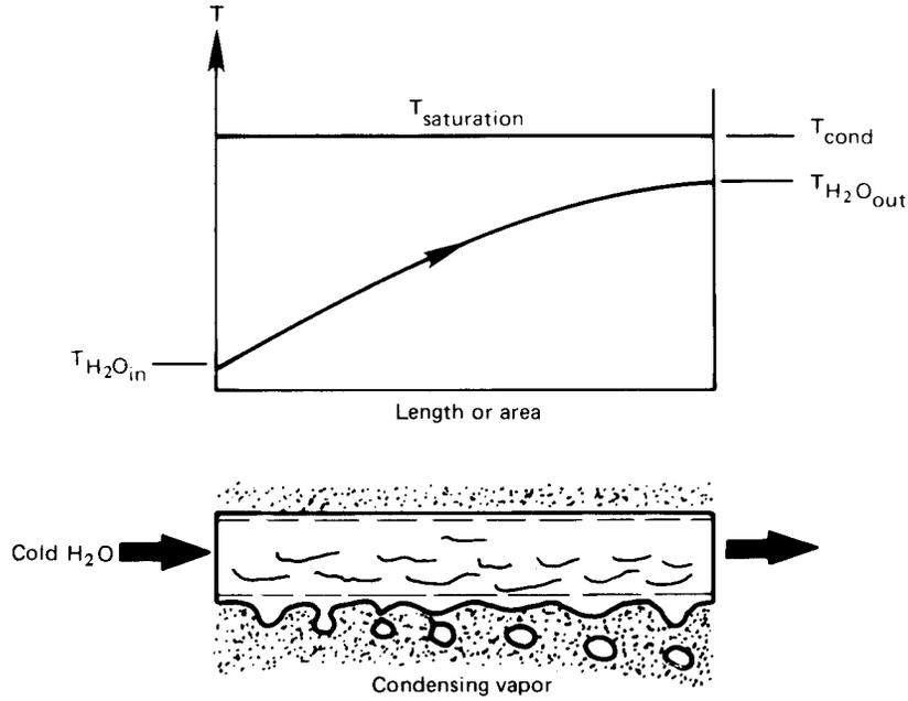
Figure 3.9 The temperature distribution through a condenser.
