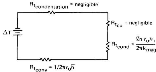
Figure 2.15 Thermal circuit for an insulated tube.
