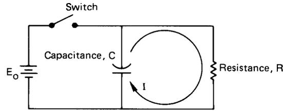
**Figure 5.1** A simple resistance-capacitance circuit.
