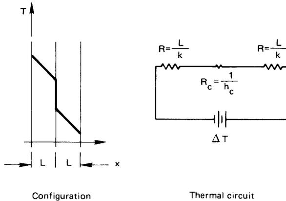
**Figure 2.11** Conduction through two unit-area slabs with a contact resistance.
