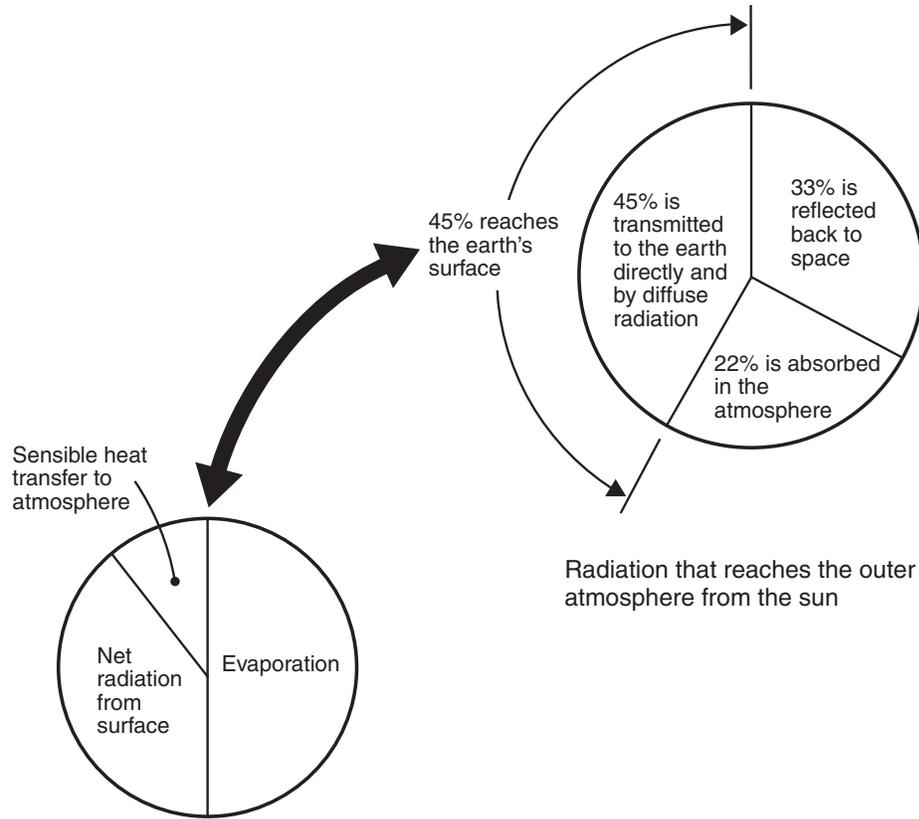
The flow of energy from the earth's surface back to - and through - the earth's atmosphere
