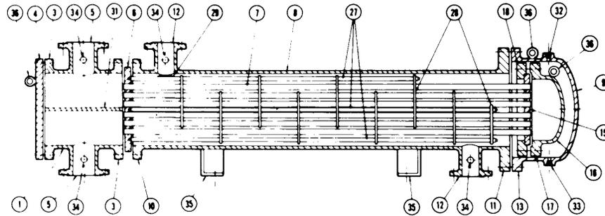
b) One shell-pass, two tube-pass exchanger
