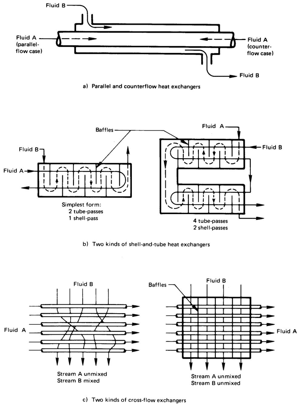
Figure 3.3 The three basic types of heat exchangers.
