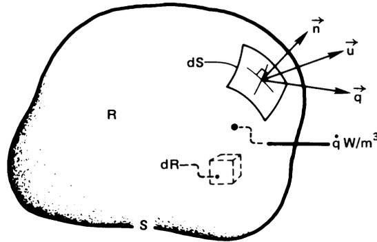
**Figure 6.12** Control volume in a heat-flow and fluid-flow field.
