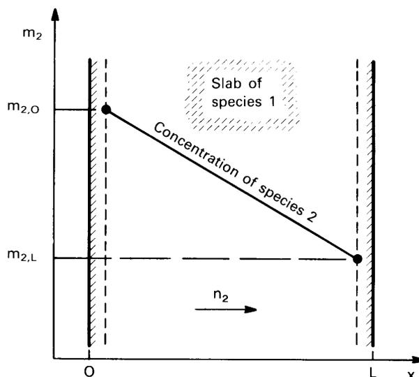
**Figure 11.12** One-dimensional, steady diffusion in a slab.
