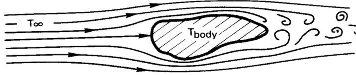
Figure 1.9 The convective cooling of a heated body.
