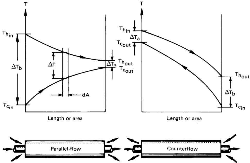
**Figure 3.8** The temperature variation through single-pass heat exchangers.
