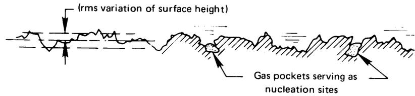
Figure 9.4 Enlarged sketch of a typical metal surface.
