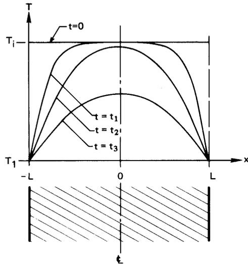
**Figure 5.6** The transient cooling of a slab;  $\xi = (x/L) + 1$ .
