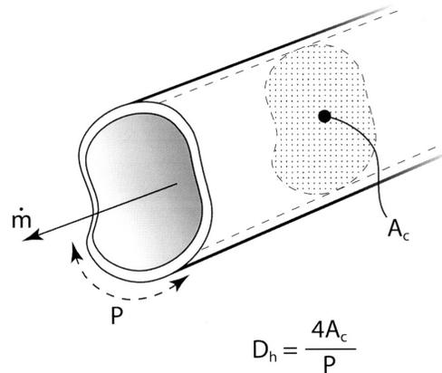
Figure 7.9 Flow in a noncircular duct.
