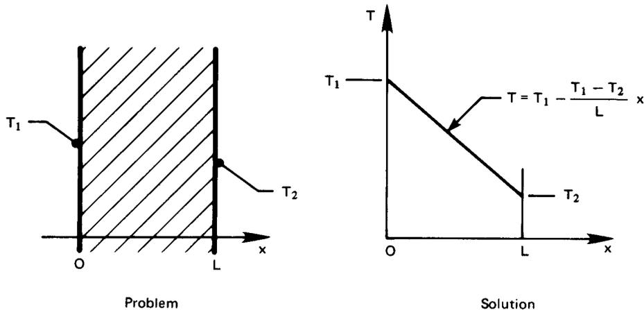
Figure 2.7 Heat conduction in a slab (Example 2.2).
