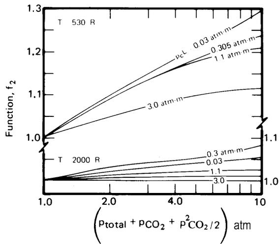
**Figure 10.23** Functions used to predict  $\epsilon_g = f_1 f_2$  for CO<sub>2</sub> in air. All pressures in atmospheres.
