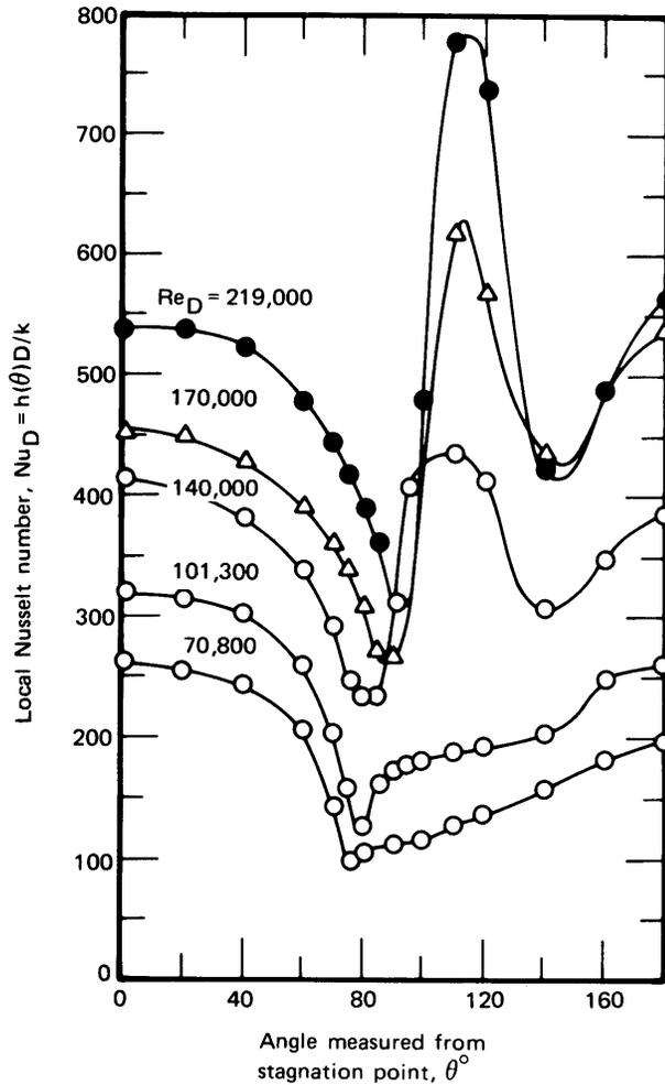
**Figure 7.12** Giedt's local measurements of heat transfer around a cylinder in a normal cross flow of air.
