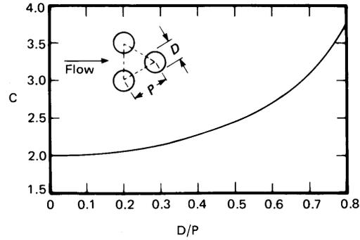
**Figure 7.17** Geometric correction for the Kalish-Dwyer equation (7.72).
