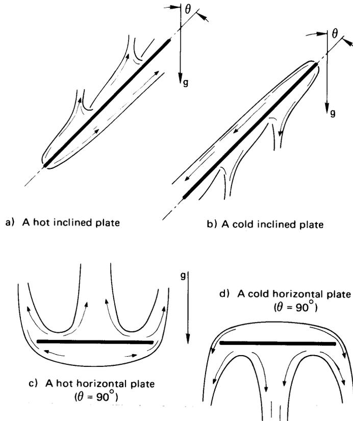
**Figure 8.8** Natural convection b.l.'s on some inclined and horizontal surfaces. The b.l. separation, shown here for the unstable cases in (a) and (b), occurs only at sufficiently large values of  $Gr$ .
