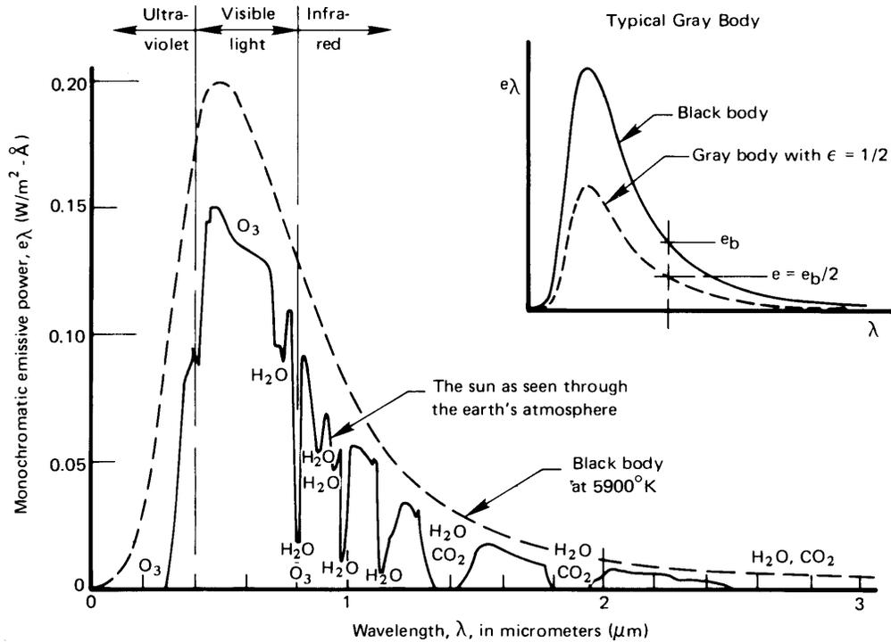
**Figure 10.2** Comparison of the sun's energy as typically seen through the earth's atmosphere with that of a black body having the same mean temperature, size, and distance from the earth. (Notice that  $e_\lambda$ , just outside the earth's atmosphere, is far less than on the surface of the sun because the radiation has spread out over a much greater area.)
