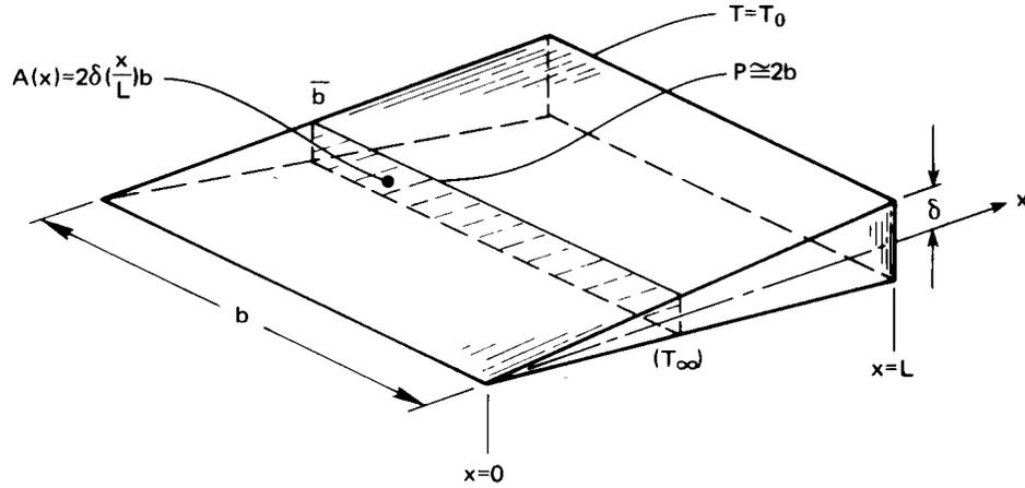
Figure 4.12 A two-dimensional wedge-shaped fin.
