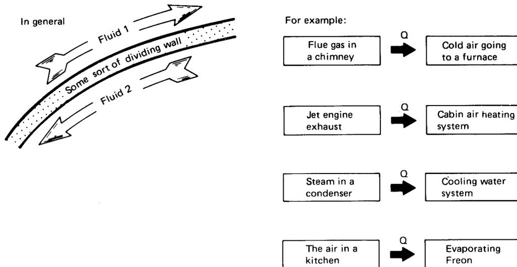
Figure 3.1 Heat exchange.
