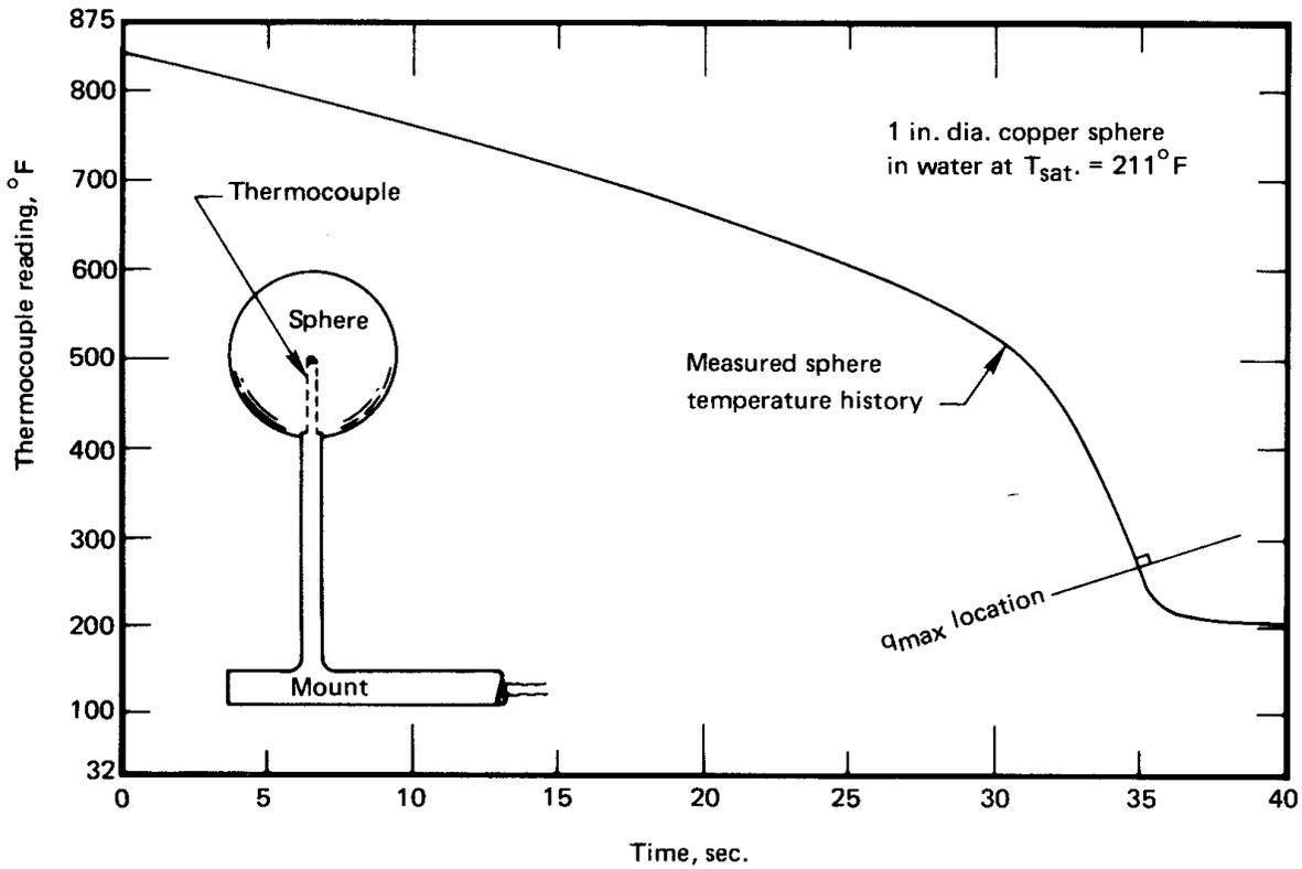
**Figure 5.28** Configuration and temperature response for Problem 5.6
