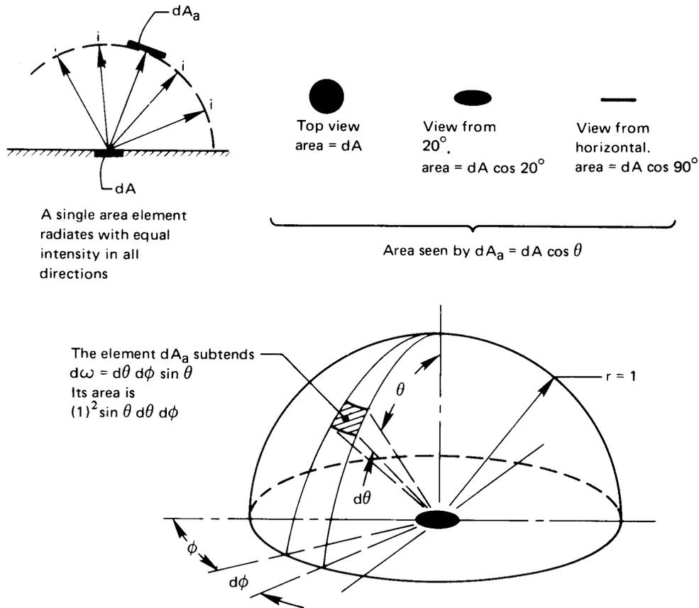
Figure 10.4 Radiation intensity through a unit sphere.
