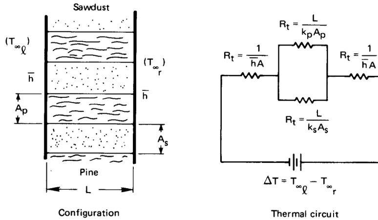
Figure 2.20 Heat transfer through a composite wall.
