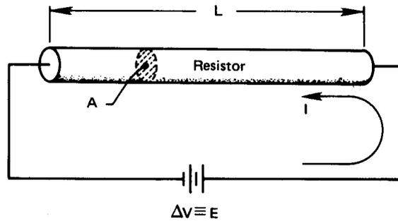
**Figure 2.9** The one-dimensional flow of current.
