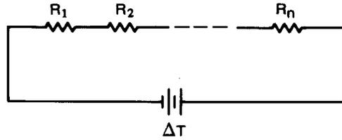
**Figure 2.18** A thermal circuit with many resistances in series. The equivalent resistance is  $R_{t_{\text{equiv}}} = \sum_i R_i$ .
