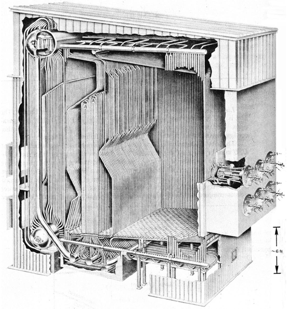
**Figure 3.12** The heat exchange surface for a steam generator. This PFT-type integral-furnace boiler, with a surface area of 4560 m<sup>2</sup>, is not particularly large. About 88% of the area is in the furnace tubing and 12% is in the boiler (Photograph courtesy of Babcock and Wilcox Co.)
