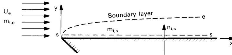
Figure 11.14 Concentration boundary layer on a flat plate.
