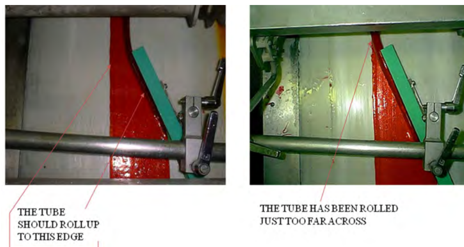
Figure 19.8. Incorrect plough set-up
