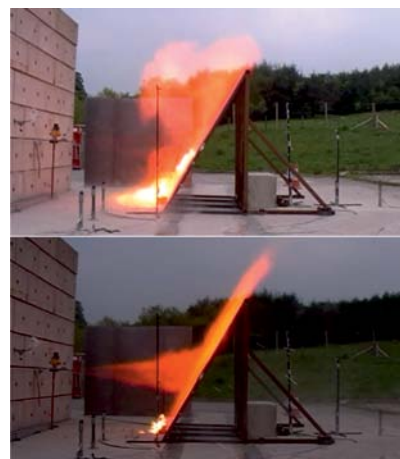
Figure 9-18. The delayed (0.8 s) ignition of hydrogen jet (20.5 MPa pressure storage, 9.5 mm diameter nozzle) impinging a 60° barrier: deflagration stage (top snapshot), steady-state impinging jet fire stage (bottom snapshot), HSL test (HYPER, 2008).
