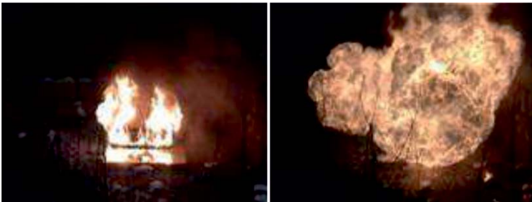
Figure 1–3. A HFCV gasoline pool fire test: (left) – gasoline fire just before initiation of TPRD, (right) – 1 second after TPRD initiation (Tamura et al., 2011).
